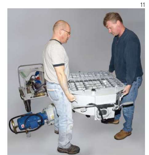
The single parts can be carried by two people without difficulty to the required location on the construction site.
