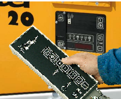
You can operate the SP 20 entirely from one side, or using the convenient radio remote control.
