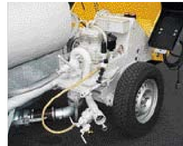
Motor, piston pump and compressor are all readily accessible beneath the raised canopy.
