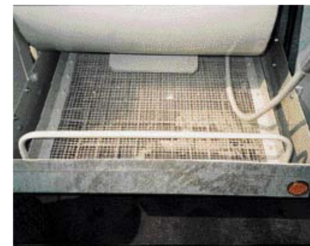
The screen features a mechanical vibratory drive installed in the galvanized mortar storage hopper. It may be removed for cleaning.
