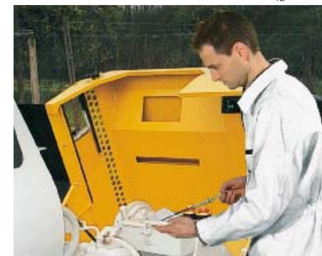
The P 13 is one of the low-maintenance plastering machines. Servicing the machine is done in next to no time as the few wearing parts can be quickly replaced.
