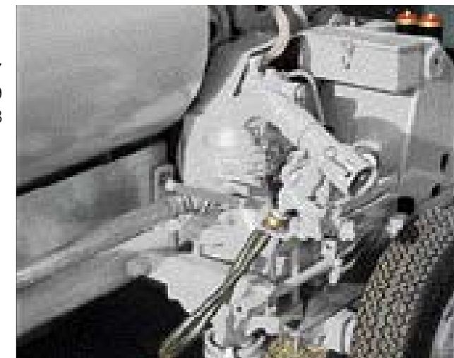
The double-piston pump (here the KK 139 with up to 120 l/ min pump output) means pulsation-free operation of the spray gun.
