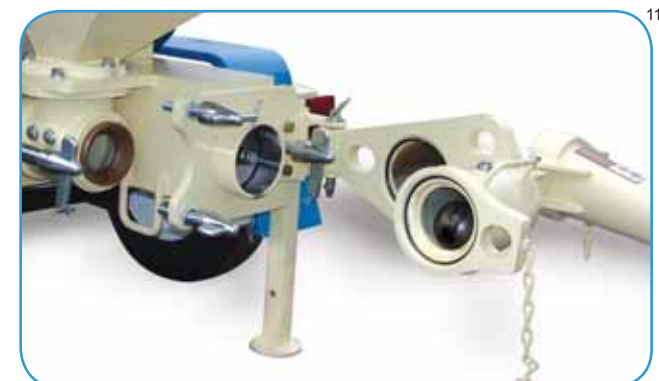
Wedge-style manifold design with fixed stop pins swings open for service.
